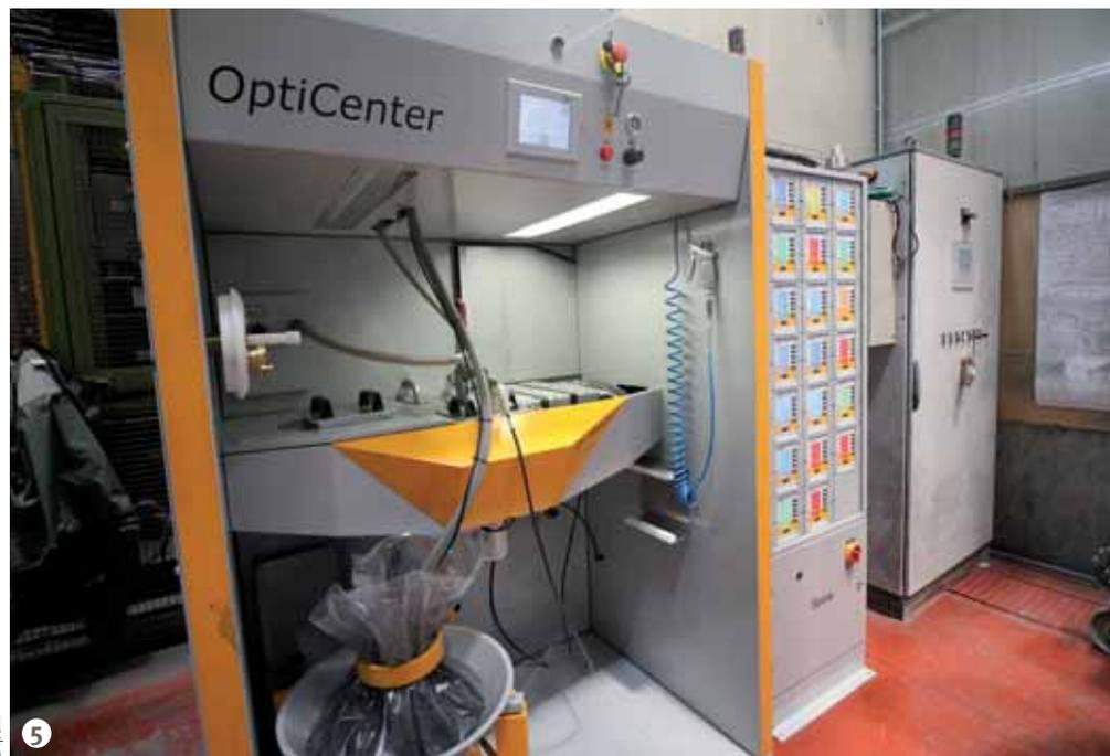
**Figure 5: Gema’s OptiCenter OC03 powder management unit.**
