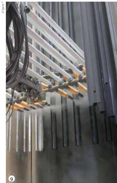
**Figure 9: The new booth's 20 guns are divided into two groups of 10 guns each: each block has 5 guns with SuperCorona parameters and 5 guns with different parameters.**
