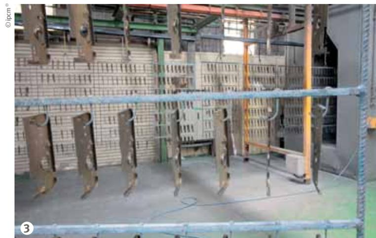
**Figure 3: Thanks to its multi-metal pre-treatment process, the highly versatile horizontal plant can coat both steel and aluminium and treat up to 8.5 m long workpieces.**
