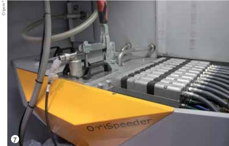
**Figure 7: OptiSpeeder is an innovative reservoir that prevents any loss due to the fluidification of powders. The closed-loop system is fully automatic, ensuring extremely low powder consumption and excellent coating results.**
