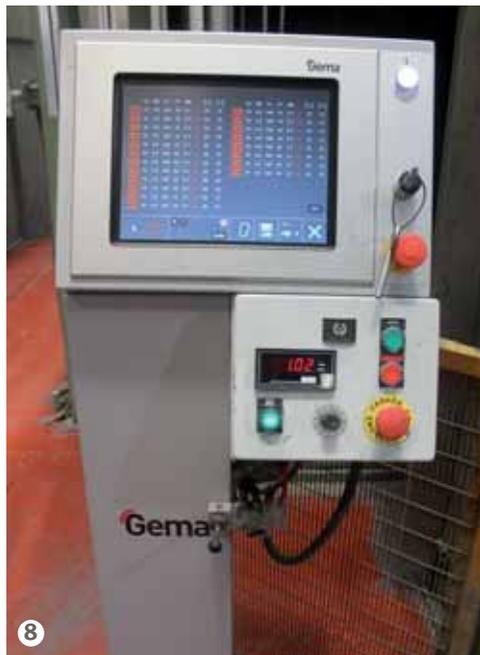
**Figure 8: The touch screen system controlling the application parameters of each gun.**
