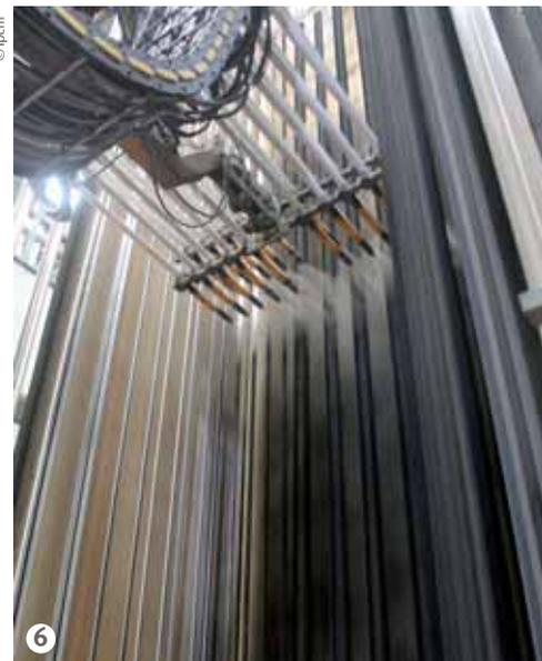
**Figure 6: The second last-generation booth supplied by SAT Spa (Verona, Italy) is U-shaped and has a quick colour change system.**
