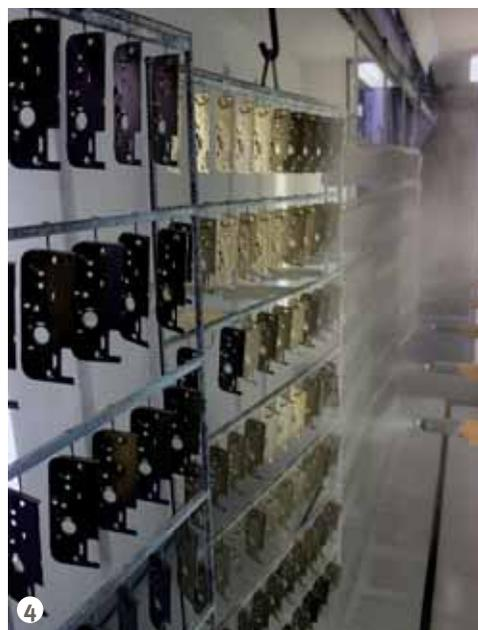
**Figure 4: The newly installed automatic booth implements several technical innovations such as automatic mixing of virgin and recovered powder and automatic recognition of the parts’ size.**
